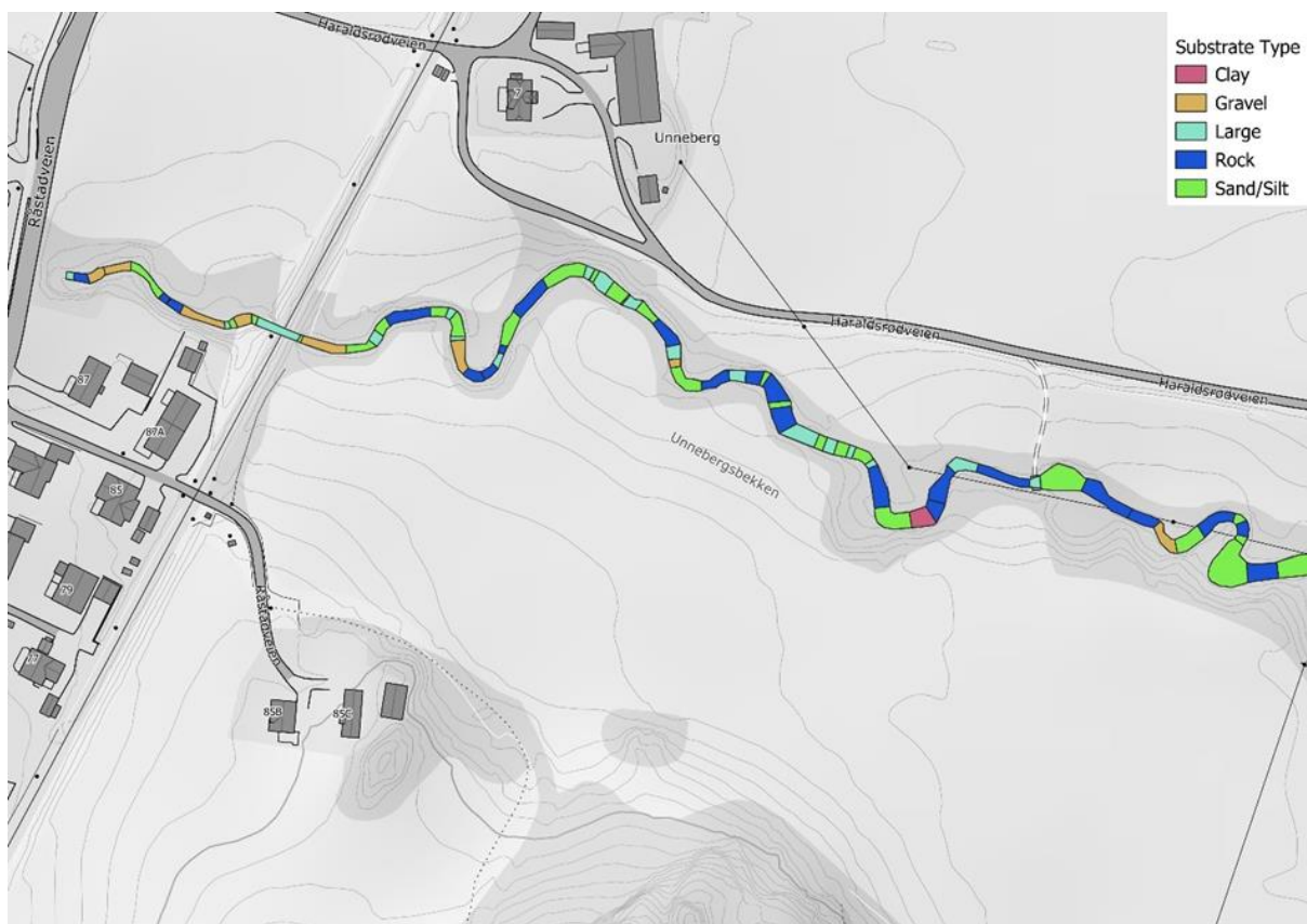
Figure 6. Example of substrate mapping in Unnebergbekken. All physical mapping followed the same procedure.
