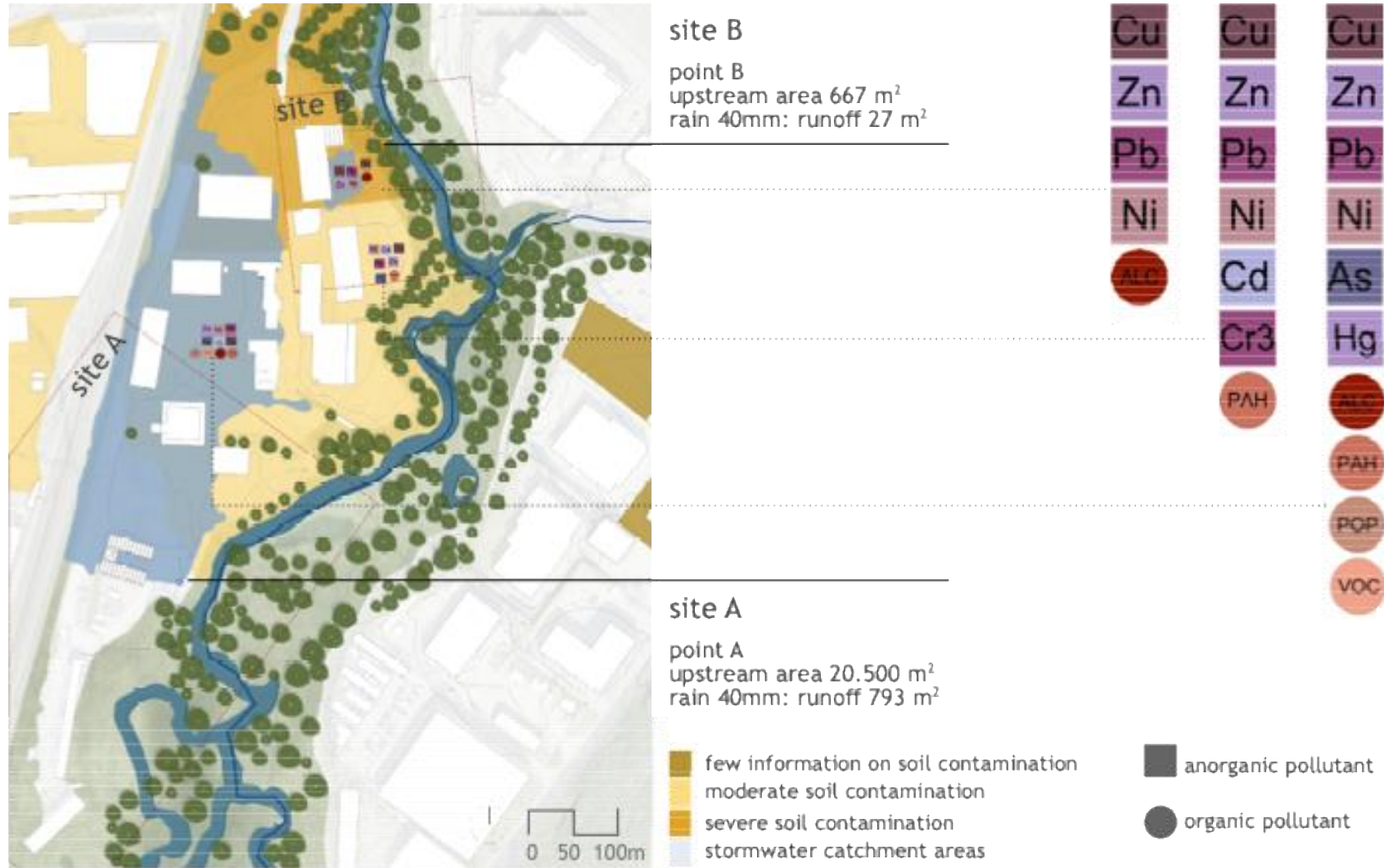
FIG.09: ANALYSIS OF CONTAMINATED GROUND AND FLOOD PATHS
