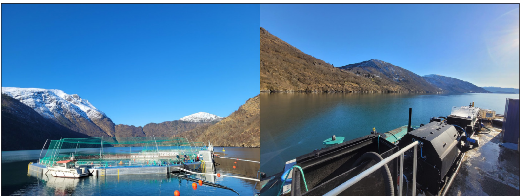
Ecomerd closed containment system in production at a Mowi site in Matersfjorden (left). The LiftUP sludge collection system on the barge (right). Foto: Sara Calabrese (NIVA)
