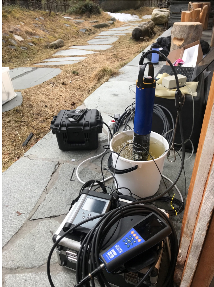
YSI Multiparameter sensor (including both FDOM and O2)
