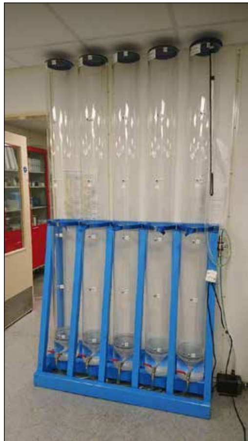
Figure 3. Water columns for instant dissolution test of freshwater liming materials.
