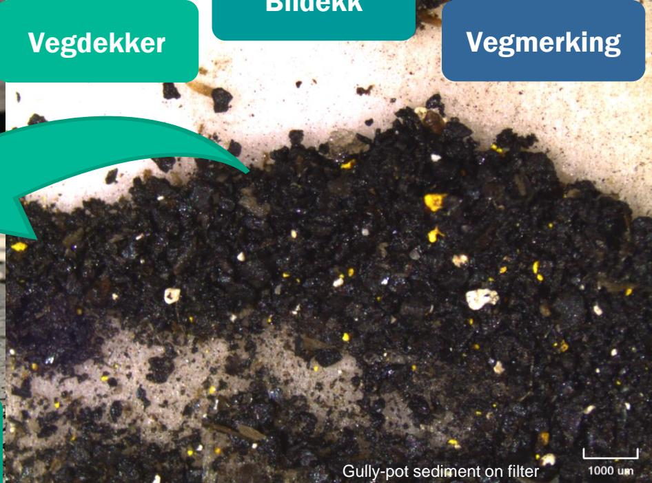
Gully-pot sediment on filter
