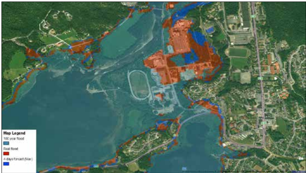
Figure 6. Flood inundation maps for the 2 nd of October 2017: 100-year return period, real flood and maximum 4 days forecast flood.
