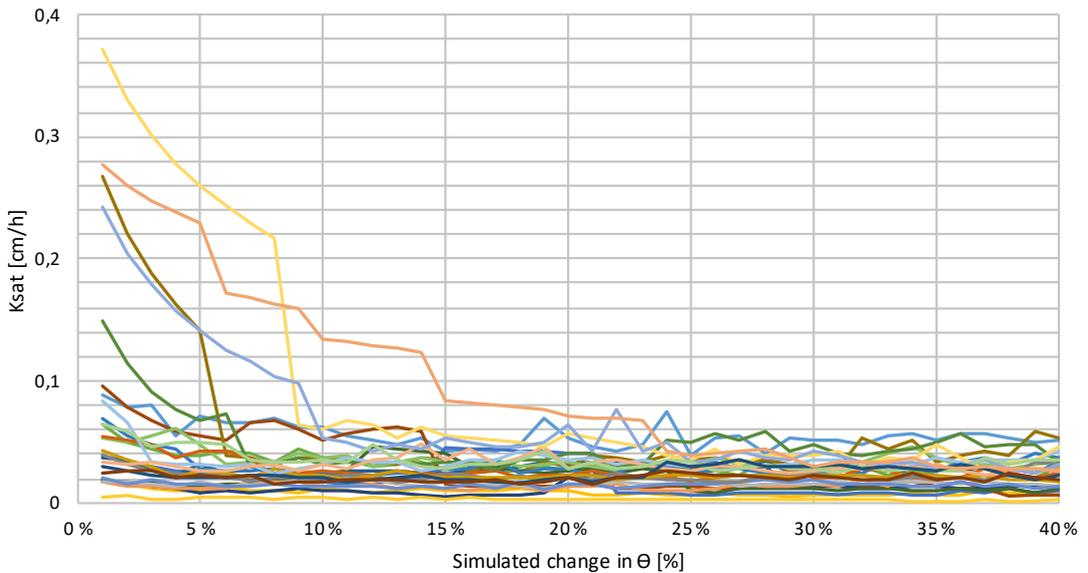
Figure 5 Simulated effect of increased change in mass water content ( $\theta$ ) during testing on field measurements of  $K_{sat}$  with theoretical highest  $K_{sat}$  above and below 0.1 cm/h.
