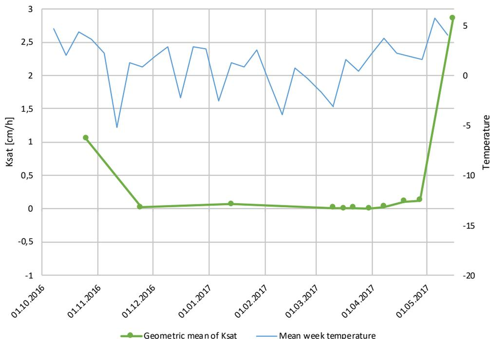
Figure 3 The variation in the geometric mean of the  $K_{sat}$  field measurements and temperature in the period of field measurements. The markers on “the geometric mean of  $K_{sat}$ ” represents the geometric mean of every usable field measurement of  $K_{sat}$  on that specified day.
