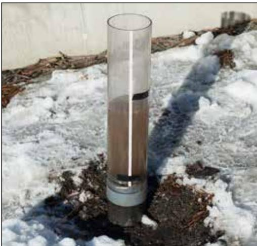
Figure 2 Picture of the Balstad Modified Philip-Dunne Infiltrometers (BMPD) column during field measurements in Mars 2016.
