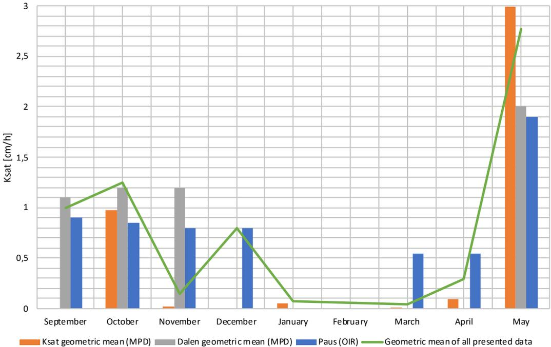
Figure 4 Comparison of this study's geometric mean  $K_{sat}$  field measurements with MPD against the geometric mean  $K_{sat}$  field measurements with MPD of Dalen (2012) and the mean  $K_{sat}$  values estimated by Paus et al. (2015) from observed infiltration rate (OIR).
