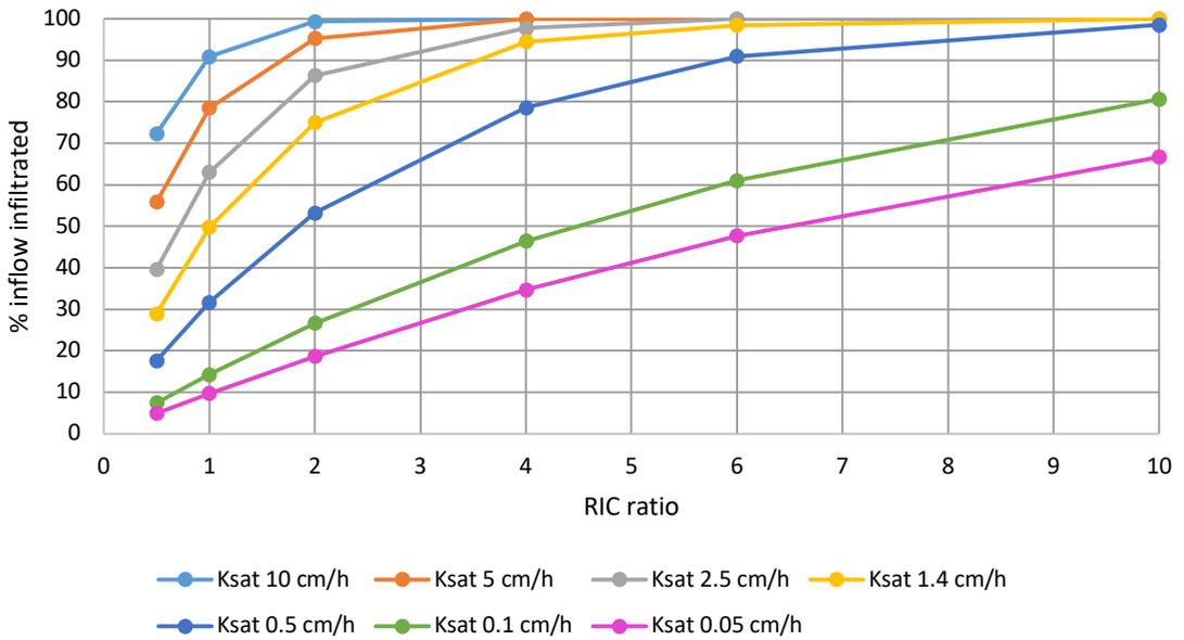
Figure 6. The effect of the raingardens infiltration capacity ( $K_{sat}$ ) and the raingarden area to impervious catchment area (RIC) ratio on the percentage of winter season inflow infiltrated. The arrow shows change in percentage of winter season inflow infiltrated, when  $K_{sat}$  changes from 1 cm/h to 0.05 cm/h.
