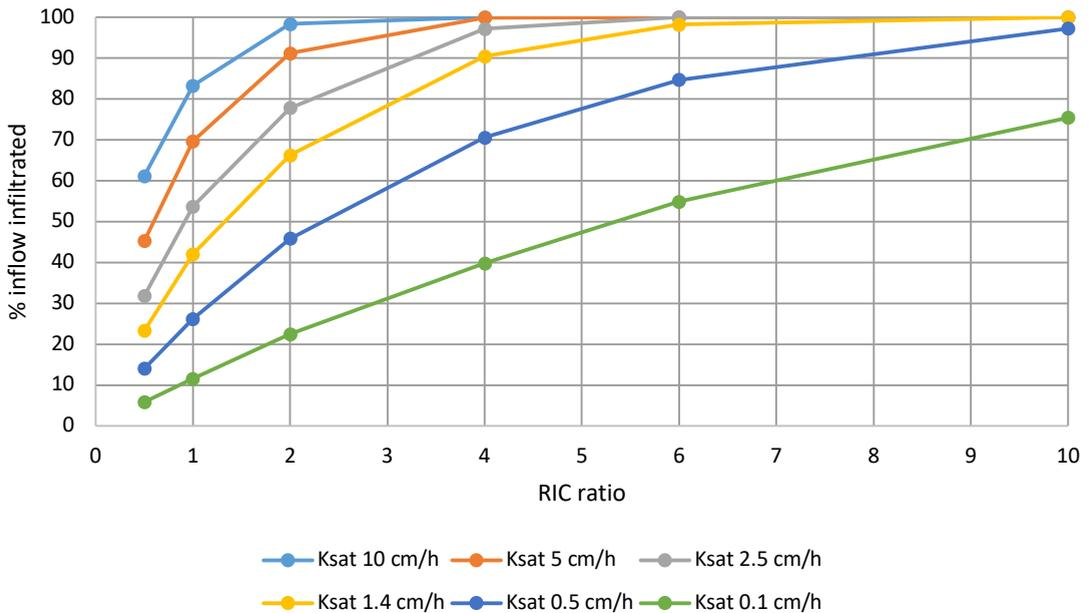
Figure 7. The effect of the raingardens infiltration capacity ( $K_{sat}$ ) and the raingarden area impervious catchment area (RIC) ratio on the percentage of summer season inflow infiltrated.
