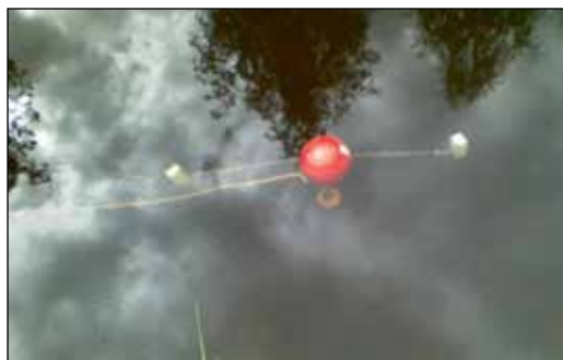
Figure 6. the passive sampling device. The red buoy was used in order to mark the device. One either side of the buoy is the POM passive sampler and the DGT.
