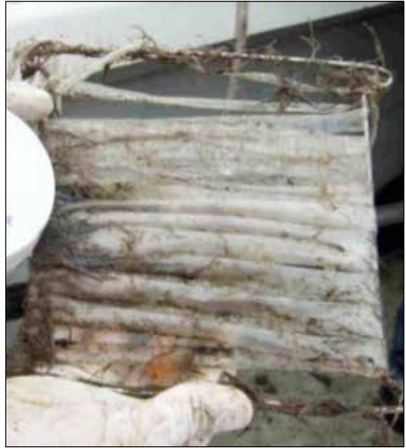
Figure 4. Photographs of the polyoxymethylene passive sampler devices used to measure the air and water PAH and PCB concentrations, respectively.
