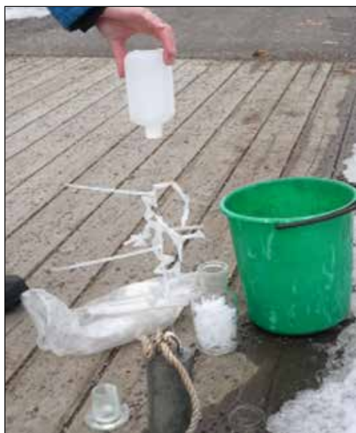
Figure 3. The polyoxymethylene passive sampling device used to measure PAHs and PCBs in the inner Oslo fjord.
