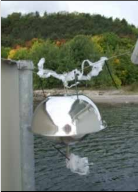
Figure 4. Photographs of the polyoxymethylene passive sampler devices used to measure the air and water PAH and PCB concentrations, respectively.
