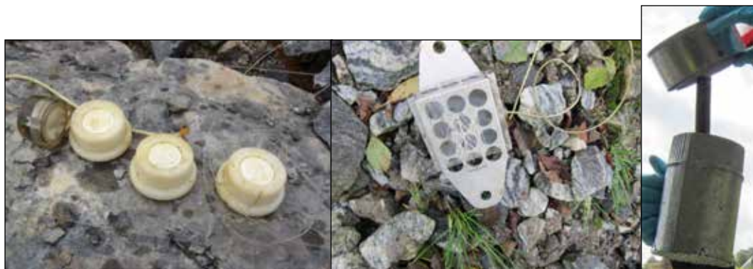
Figure 2. The passive sampling devices used in the WASTEFFECT project. From left to right; DGT used to sample Sb, polydimethylsiloxane and polyoxymethylene used to sample BFRs and BPA, respectively, in water (both membrane materials are encapsulated in a stainless steel cage) and XAD beads (contained in the tube which is protected by the stainless steel cage).
