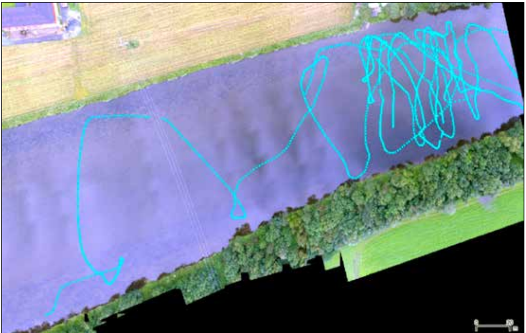
Figure 8. Artefacts in the mosaic image for Svean caused by strong cloud reflections.
