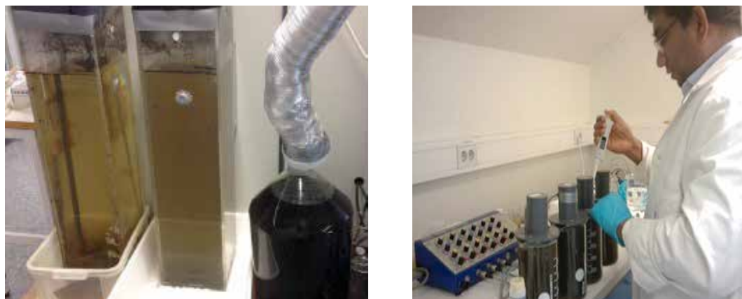
e) Two aerobic and one anaerobic test vessels (left picture); f) Chemical precipitation tests using Jar-tests (right picture).
