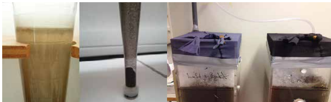
c) The sedimentation lab-test with Imhoff glass (left picture); d) Aerobic biodegradation (right picture).
