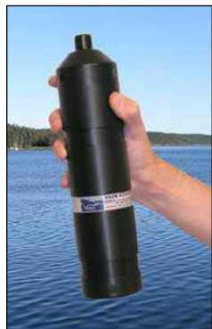
Figure 5: A VR2w receiver for passive monitoring of tagged sea trout (Photo credit: www.Vemco.com )
